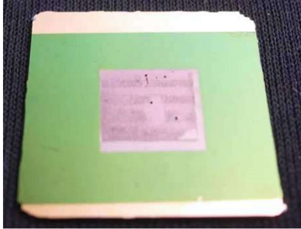
Fig. 57 The whole photograph of FPA pixel at size of 57 \times 57 \mu\text{m}^2
