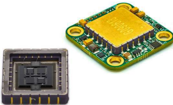
Fig. 41 Wire bonding of the sensing element in the ceramic package and the completed device with readout circuit
