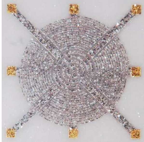
Fig. 29 Micrograph of the wind sensor fabricated on ceramic substrate
