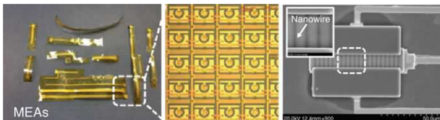
Fig. 4 Photo of MEA with silicon-nanowire FET switches
