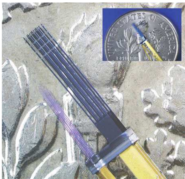
Fig. 10 Released silicon probe with parylene flexible cable and SEM picture of the electrodes on the silicon shanks
