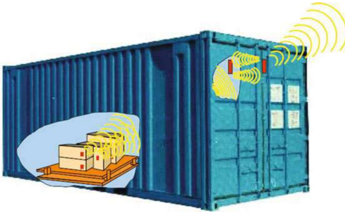
Fig. 1 Application of MEMS inertial switch in monitoring the transportation of goods
