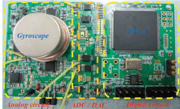
Fig. 9 The AGC + PLL control circuit for a MEMS gyroscope
